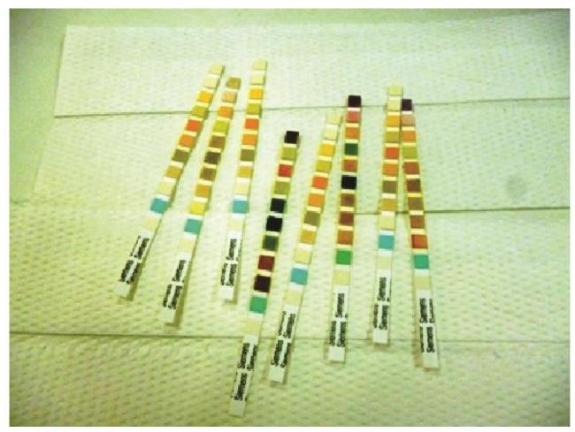
**Figure 12.4** Test strips are commonly used to detect the presence of specific substances in a person's urine. Many test strips have several pads containing various reagents to permit the detection of multiple substances on a single strip. (credit: lqbal Osman)
