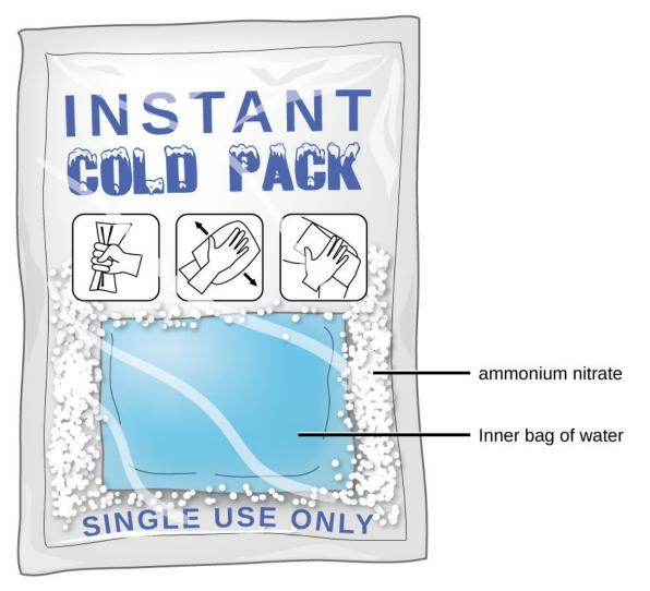
**Figure 11.4** An instant cold pack gets cold when certain salts, such as ammonium nitrate, dissolve in water—an endothermic process.
