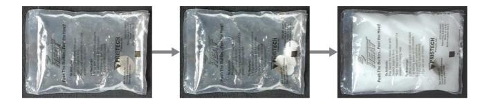
**Figure 11.10** This hand warmer produces heat when the sodium acetate in a supersaturated solution precipitates. Precipitation of the solute is initiated by a mechanical shockwave generated when the flexible metal disk within the solution is "clicked." (credit: modification of work by "Velela"/Wikimedia Commons)
