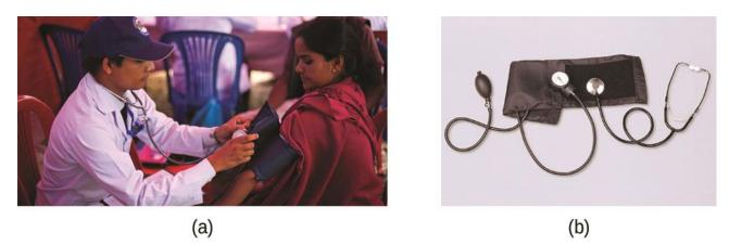
**Figure 9.5** (a) A medical technician prepares to measure a patient's blood pressure with a sphygmomanometer. (b) A typical sphygmomanometer uses a valved rubber bulb to inflate the cuff and a diaphragm gauge to measure pressure. (credit a: modification of work by Master Sgt. Jeffrey Allen)
