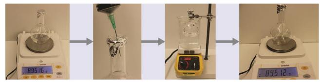
**Figure 9.22** When the volatile liquid in the flask is heated past its boiling point, it becomes gas and drives air out of the flask. At  $t_{1\rightarrow g}$ , the flask is filled with volatile liquid gas at the same pressure as the atmosphere. If the flask is then cooled to room temperature, the gas condenses and the mass of the gas that filled the flask, and is now liquid, can be measured. (credit: modification of work by Mark Ott)
