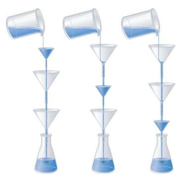
**Figure 12.16** Rate-determining step. The phenomenon of a rate-determining step can be compared to a succession of funnels. The smallest-diameter funnel controls the rate at which the bottle is filled, whether it is the first or the last in the series. Pouring liquid into the first funnel faster than it can drain through the smallest results in an overflow.
