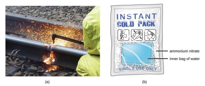
**Figure 8.8** (a) An oxyacetylene torch produces heat by the combustion of acetylene in oxygen. The energy released by this exothermic reaction heats and then melts the metal being cut. The sparks are tiny bits of the molten metal flying away. (b) A cold pack uses an endothermic process to create the sensation of cold. (credit a: modification of work by "Skatebiker"/Wikimedia commons)
