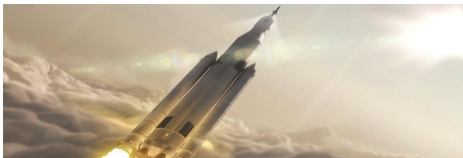
**Figure 7.1** Many modern rocket fuels are solid mixtures of substances combined in carefully measured amounts and ignited to yield a thrust-generating chemical reaction. (credit: modification of work by NASA)
