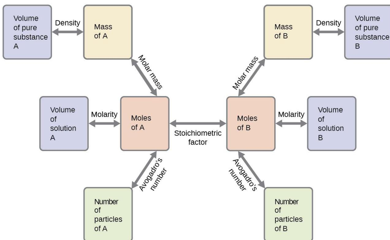
**Figure 7.5** The flowchart depicts the various computational steps involved in most reaction stoichiometry calculations. Note that you will learn more about molarity in CH 122 and CH 123.
