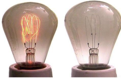
**Figure 3.8** Example of a blackbody radiation.
