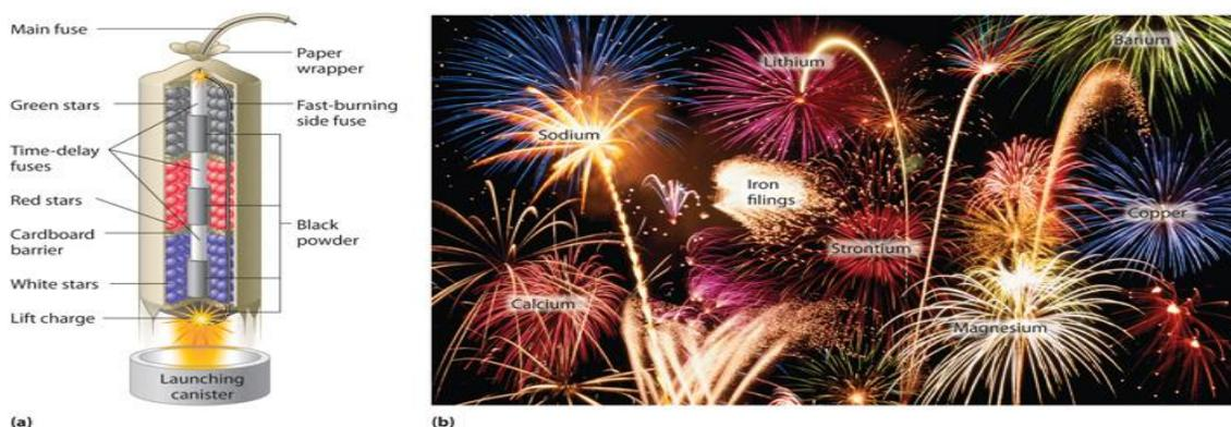
**Figure 3.16** (a) In the “multibreak” shell used for fireworks, the chambers contain mixtures of fuels and oxidizers plus compounds for special effects (“stars”) connected by time-delay fuses so that the chambers explode in stages. (b) The finale of a fireworks display usually consists of many shells fired simultaneously to give a dazzling multicolor display. The labels indicate the substances that are responsible for the colors of some of the fireworks shown.
