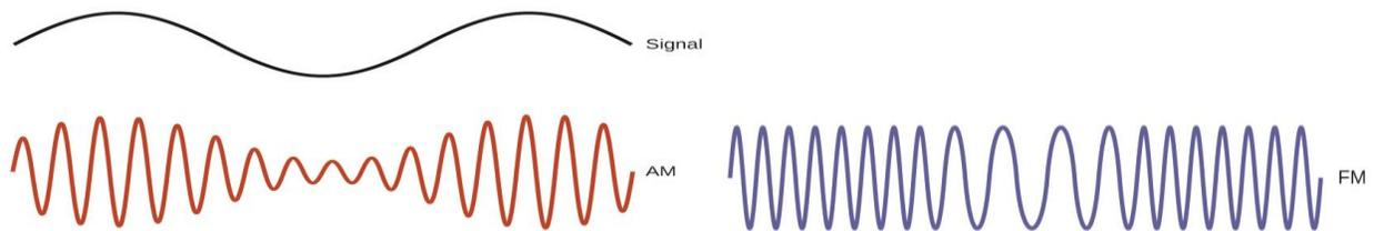
**Figure 3.5** This schematic depicts how amplitude modulation (AM) and frequency modulation (FM) can be used to transmit a radio wave.
