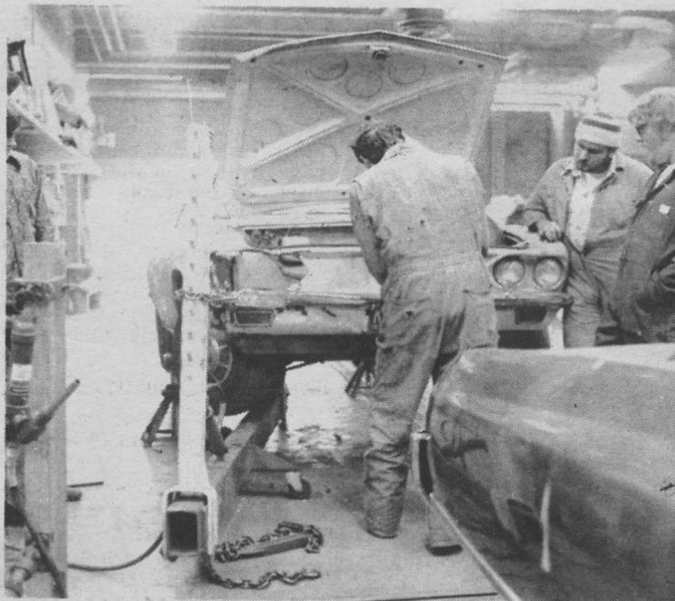
One project they are working on is the installation of a sun roof in a 4-wheel drive jeep.
