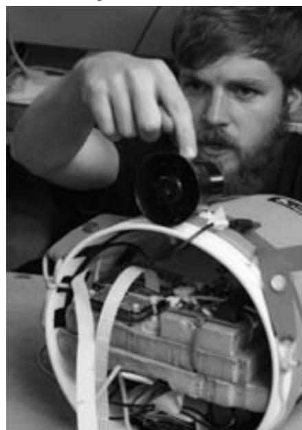
In order to ensure that the payload didn't get flooded as it landed in the ocean the team waterproofed the payload technology. They used a two-gallon bucket, painted orange to ensure that it was easily visible at sea, and insulated with Dynaflex.
