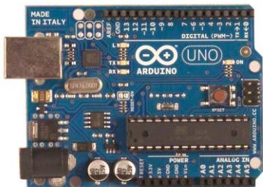
A microcontroller is a small computer on a single integrated circuit with programmable input/output peripherals. Physicists are interested in microcontrollers as these tend to be a main tool we use to collect data from the universe and to control the devices that make up our experimental apparatus.
