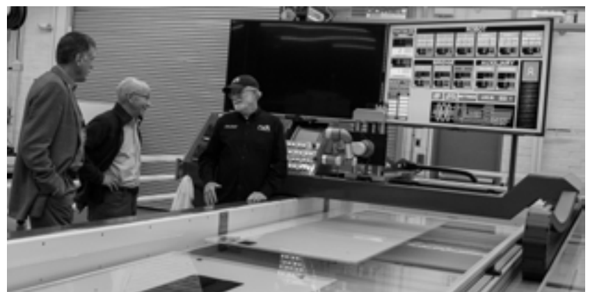
Funds from the General Obligation bond measure have gone into renovations in LBCC's CTE programs, and have helped upgrade programs such as Non-Destructive Testing, providing money for new equipment such as an immersion tank for ultrasonic testing (pictured).
