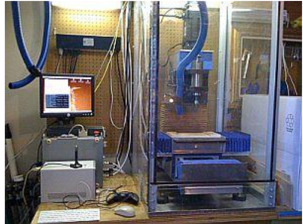
Figure 4: Our home-made milling machine, controller and enclosure constructed from parts found on Internet auction sites, surplus vendors and parts that we fabricated. Most components of the NOVA were wholly or partially created via this CNC mill.
