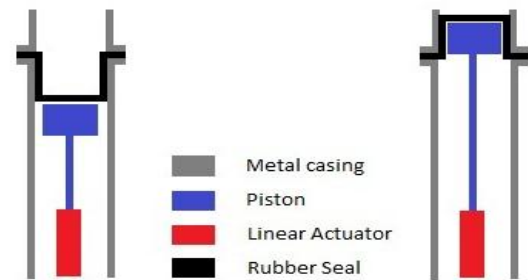
Figure 18: A diagram depicting the different stages that the variable buoyancy device goes through its process.
